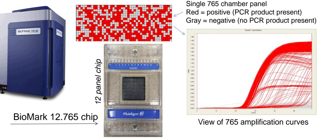
Utilizes a microfludic chip to partition the PCR mastermix into 765 chambers (volume of each chamber = 6 nL).
