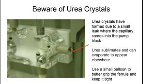
Pump block should be well cleaned to avoid problems with urea crystal formation
